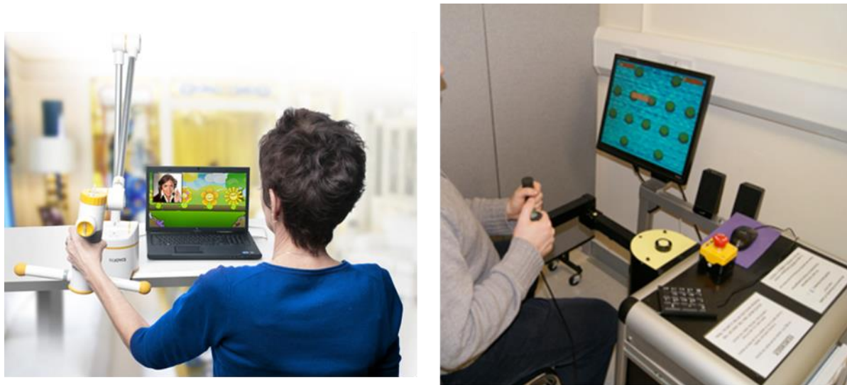
Figure 10. The ReJoyce (left) and hCAAR (right) - attempts to replicate rehabilitation robot arms for home use. [45], [46]
