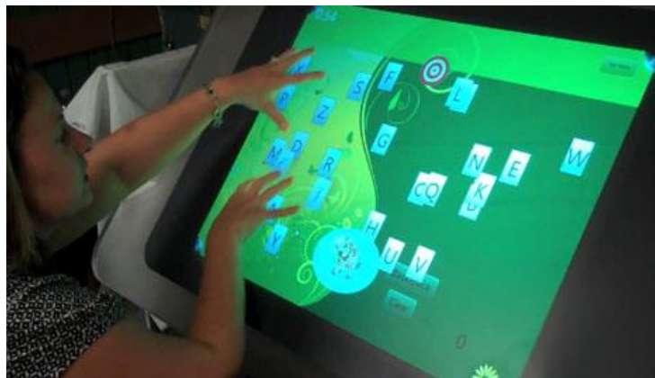
Figure 8. Spaulding touchscreen rehabilitation system. Displayed is a spelling rehab game requiring physical manipulation of letters across the screen. [4]
