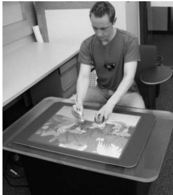
Figure 11. Passive tangibles (a wand and a ball) in use with a rehabilitation touchscreen. [4]
